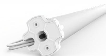
Automate Wire-Free Li-ion Q3.0 v2 5V, 3.0Nm, Ø35mm, 20-28PRM, 851mm long
