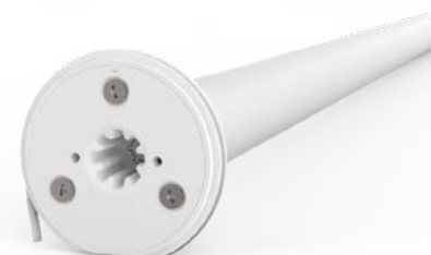
Automate Wire-Free Li-ion Zero Q1.1 5V, 1.1Nm, Ø25mm, 20-28RPM, 552mm long
