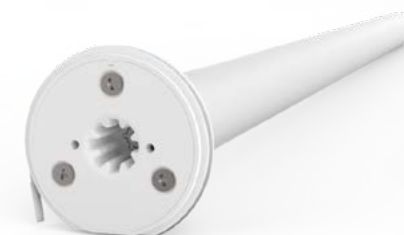
Automate Wire-Free Li-ion Zero Q1.1 5V, 1.1Nm, Ø25mm, 20-28RPM, 552mm long
